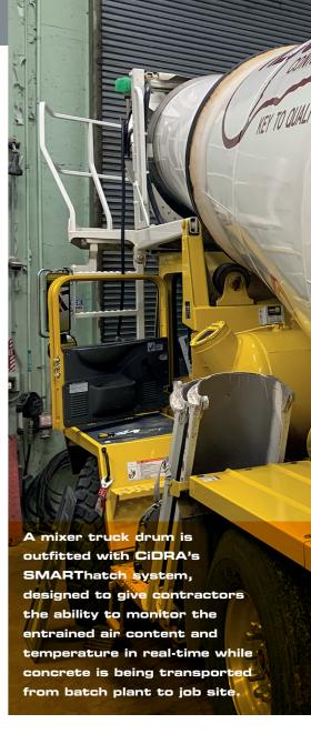
along with GPS data and other metrics, over a 4G LTE cellular interface, to a back office platform, where it can be accessed by remote users. Real time information, including concrete air content percentage, drum speed, concrete temperature and sensor battery level is also sent to a display mounted in the vehicle cab.
