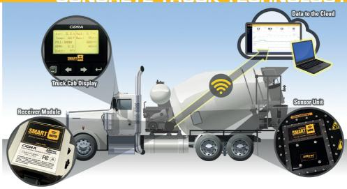
The core of the CiDRA Smarthatch system is the AirTrac system that provides non-contact measurement of entrained air and temperature of the concrete in the mixer truck drum. That information is displayed in the vehicle cab and transmitted to the cloud via HED's CANect Telematics system.
